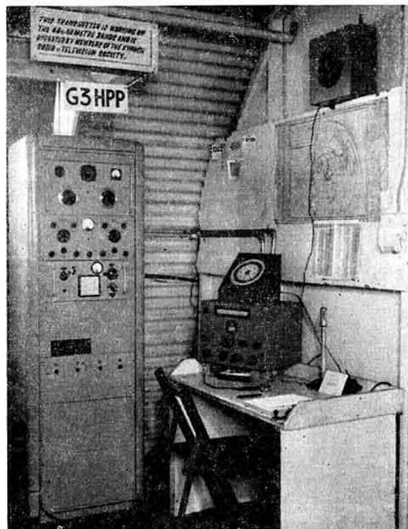
The 3.5 Mc/s station operated by members of the Kynoch Radio and Television Society under their call-sign G3HPP. The transmitter comprised a modified TU5B unit as a v.f.o. driving an 807 followed by a pair of 807s in parallel in the p.a. On the right is the modified CR100 receiver (Photo by Kynoch Press)
